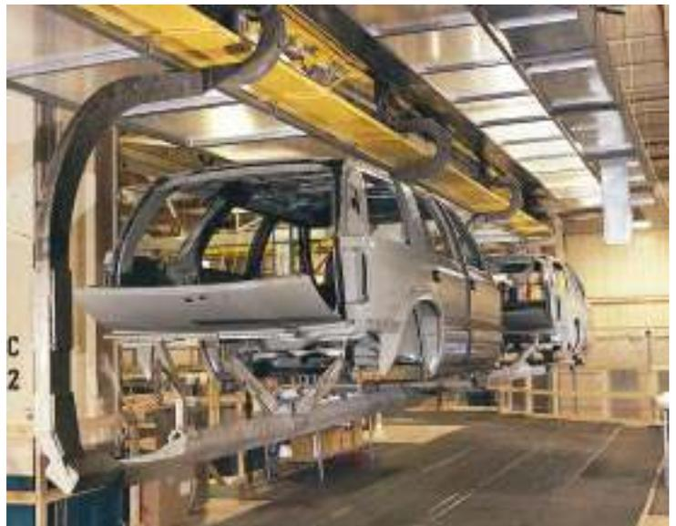
**Optimum Use of Floor Space...**Inverted Power & Free transports the product on a pedestal, therefore production line operations can be performed quickly and efficiently without obstruction. The system may be mounted on the floor, flush with the floor, or at building truss height to accommodate plant conditions.
