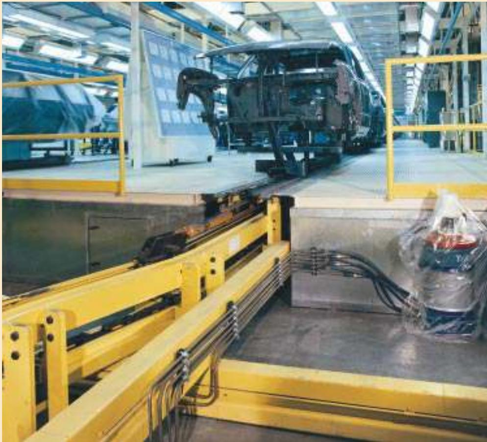
A broad range of manufacturing requirements are easily handled by Wide Wing Dog Magic Power & Free conveyors. These features allow the conveyors to interface smoothly with automatic work stations, loading and unloading equipment, and a variety of production robots.
