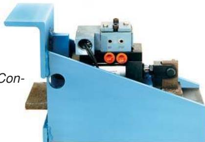
*Uni/Uni Overhead Conveyor standard stop assembly*
