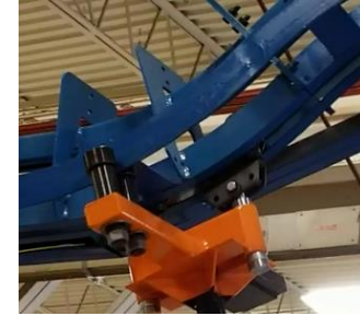
I-beam style Power and Free
