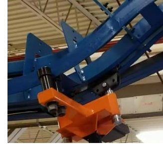
I-beam style Power and Free
