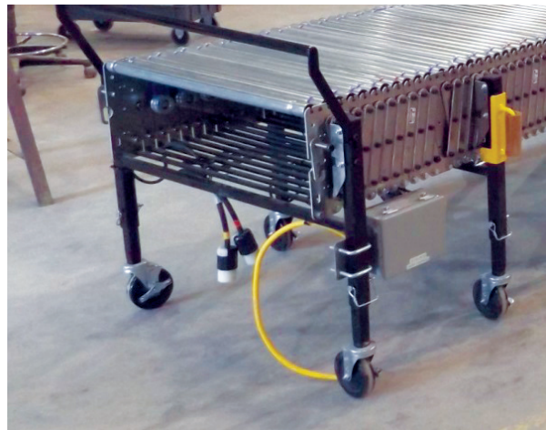
Figure 24: Powered Flex Conveyor, infeed end
